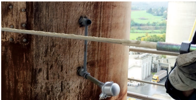
Figure 2. Dust covered sensor – its accuracy is unaffected.
