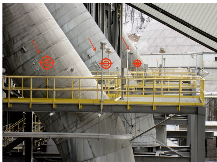
Figure 4. St Genevieve Measurement of air flows on all finished product mills.
